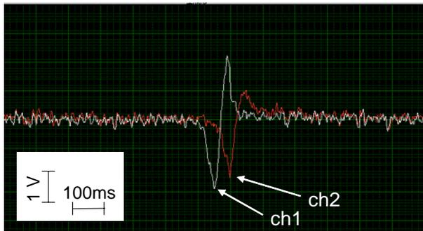
Fig. 11. Time trace of the signals from SQUIDs. Conversion factor of Volt to Tesla is 30 pT/V. Clear peaks can be seen.
