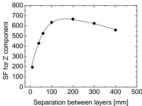
Fig. 6. Shielding factor as a function of layer separation. Shielding factor presents a non-linear behavior and maxima at around the layer separation of 100 to 200 mm.
