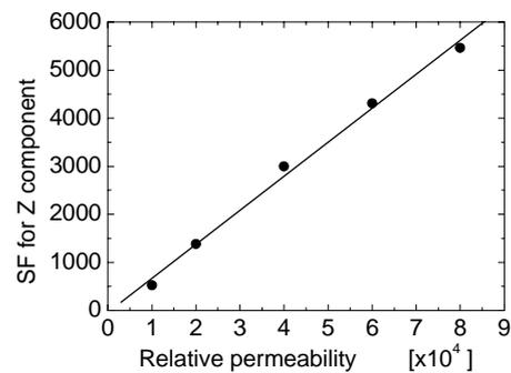
Fig. 4. Dependence of the SF on the relative permeability. It indicates that the SF increases linearly along the relative permeability  $\mu_r$ .
