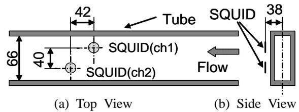
Fig. 9. Configuration of the SQUIDs. Two identical SQUIDs were employed so that they can keep the sensitivity over the full width of the tube.
