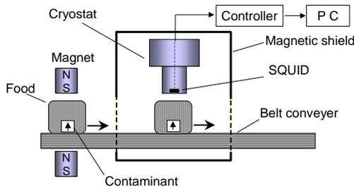
Fig. 1. Block diagram of a contaminant detection system for food.
