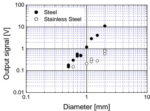
Fig. 8. Dependence of the SQUID output peak signal on the sample diameter. Conversion factor of Volt to Tesla is 1.2 nT/V.
