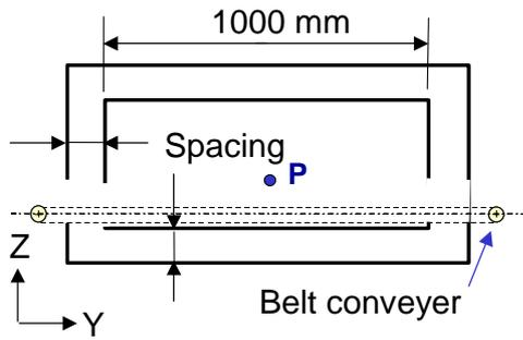
Fig. 5. Rectangular shape model for FEM simulation. This model is more realistic and suitable for the system. The number of the shield layer is two.
