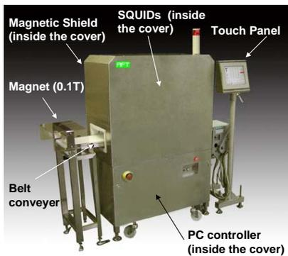
Fig. 2. Appearance of the whole system. The size of the system is 1500L mm x 477W mm x 1445H mm and is covered with stainless steel.
